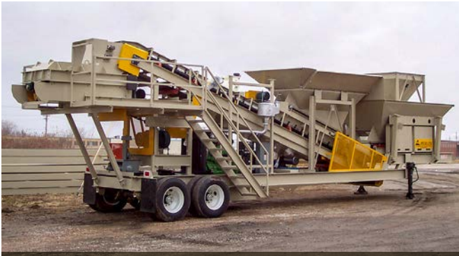
Model 950 portable pugmill plant is built with a dual feed system and cement hopper with PLC blending controls
