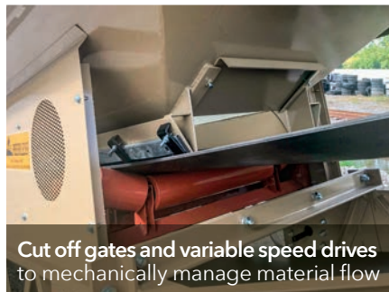
12' x 7' 13 cubic yard (struck capacity) portable high discharge feed hopper
